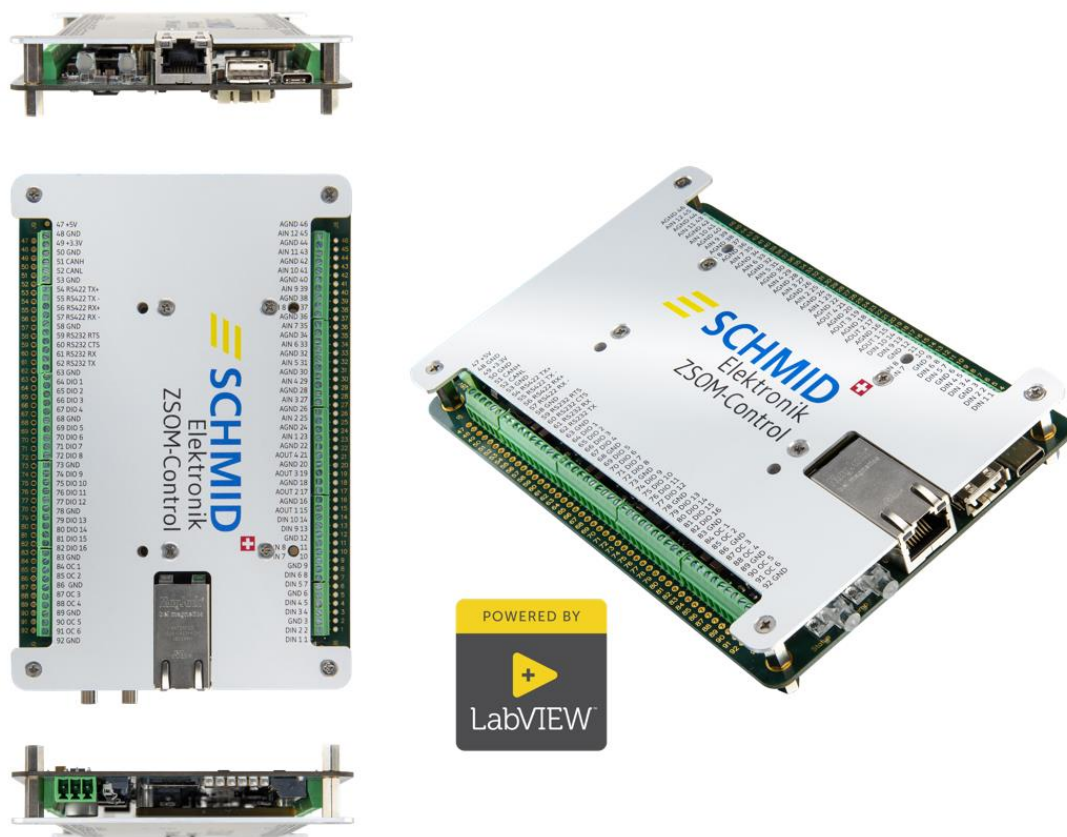
Fig.12 | The ZSOM-Control is an industrial single-board computer. The process I/O can be connected directly to robust screw terminals.
