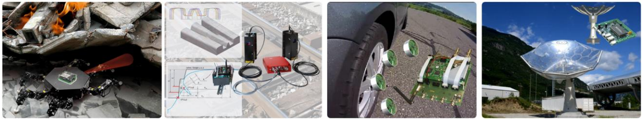
Fig.15 | Examples of Zbrain applications (from left to right): six-legged robot for disaster relief operations, monitoring the wear of railway infrastructure, measuring rotation in the wheel hub and controlling a compact and highly efficient solar power plant.
