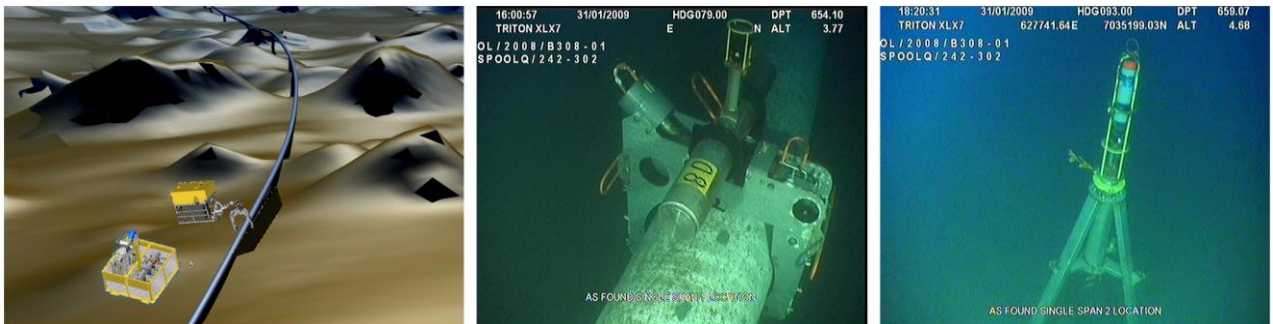
Fig. 3 | A Remote Operating Vehicle (ROV, left) anchors the CSP (Clamp Sensor Package, centre) on the pipeline and the MSP (Master Sensor Package, right) on the seabed.
