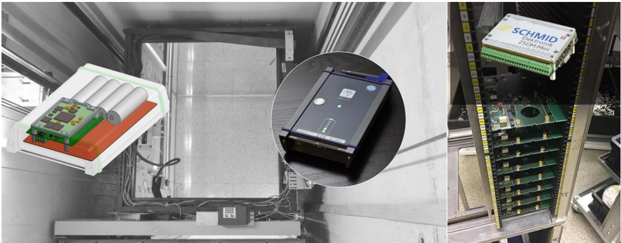
Fig. 18 | A battery-operated measuring handheld for the lift contains a high-precision acceleration sensor and communicates the data to the tablet via WIFI.
