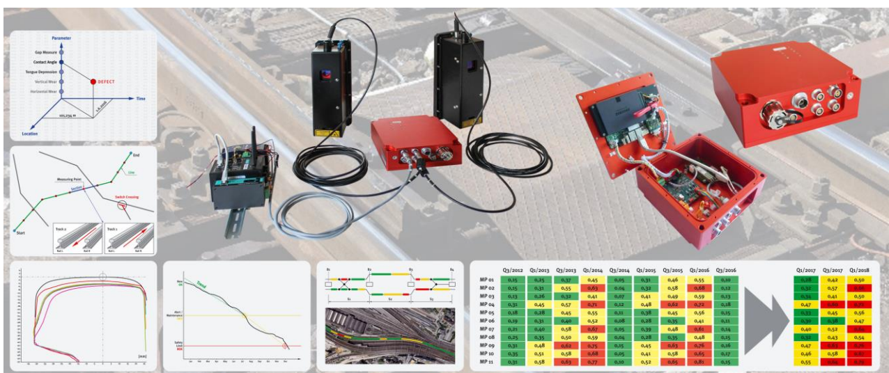
Fig. 6 | Laser-based, automated condition monitoring of railway track infrastructure: two laser scanners (black) are connected to the main computer (red) and are controlled by LabVIEW Embedded. The measurement data is stored in a structured manner according to a network plan, processed and made accessible to everyone at the appropriate level.
