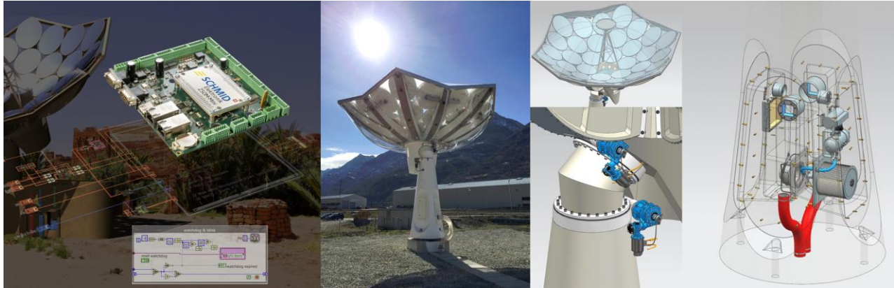
Fig. 8 | A vision for the highly efficient solar energy of tomorrow with a complex mix of technologies: from the rough concrete structure to the micromechanical silicon cooling system, with a graphically programmable embedded system with safety and emergency functions, IoT-Link and local measuring network with over 100 controlled sensors and actuators on the CAN bus.
